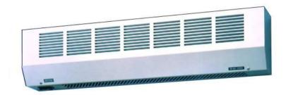
This heater appliance is intended for use as a warm air curtain and is to be mounted on the wall above doorways or along a wall. It is to be mounted with the underside a maximum of 2.1 metres above floor level. It can be mounted directly to a wall surface to provide a near vertically downward air discharge or on angled mounting brackets (supplied) to provide an air discharge angled 25° from downward. If exceeding 3 metres there will be a reduction in performance.
